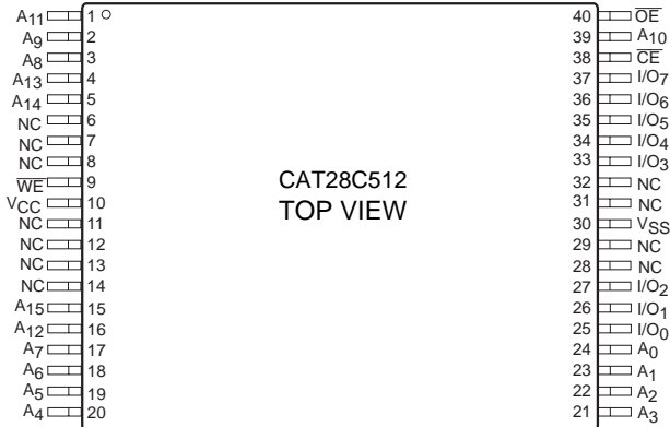
TSOP Package (10mm X 14mm) (T14)
